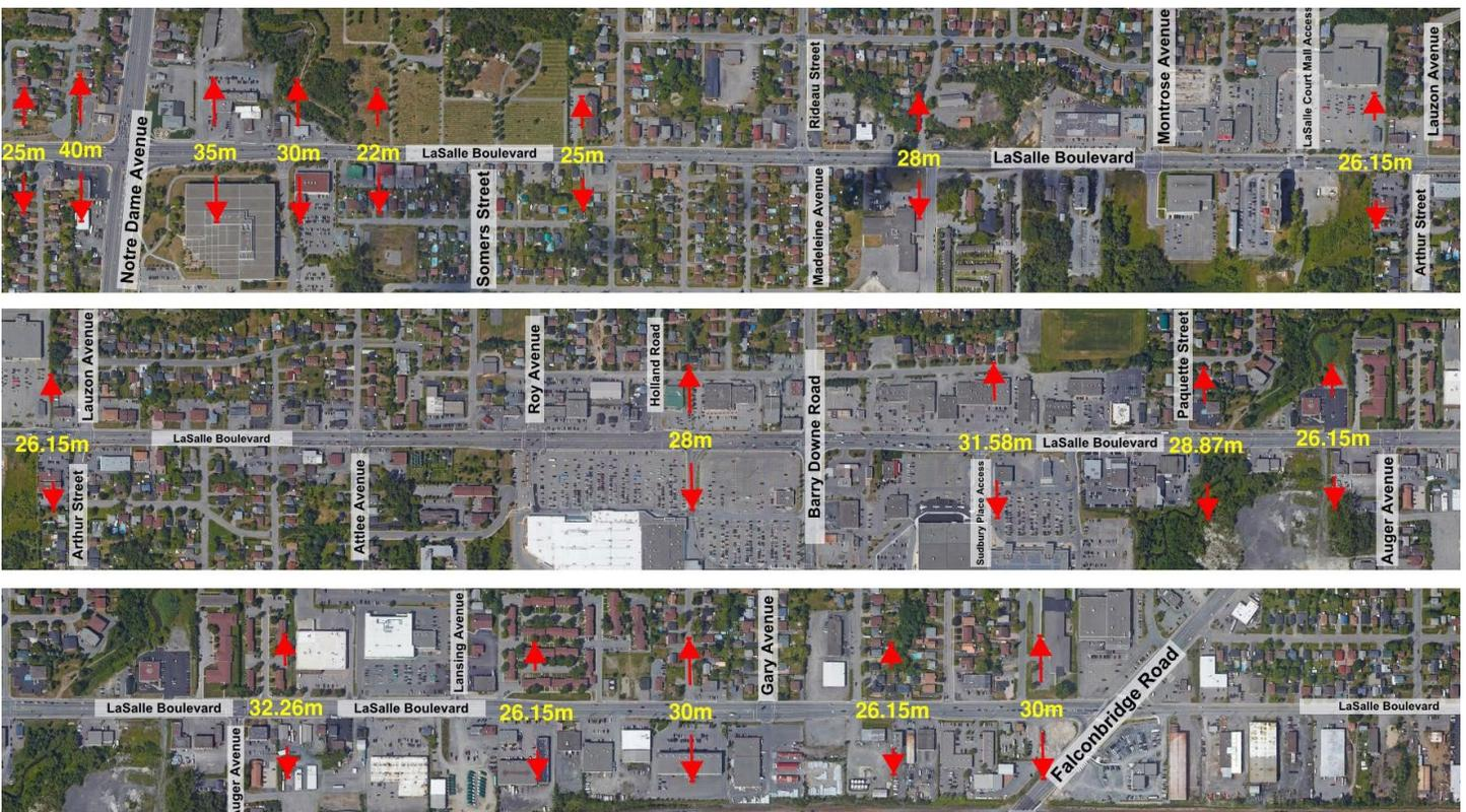
Figure 5: Right-of-Way (ROW) Widths
