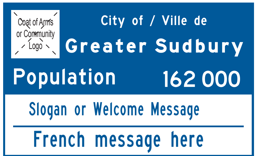
G315 (B) (2100 mm x Variable Width) - Two piece plywood sign
