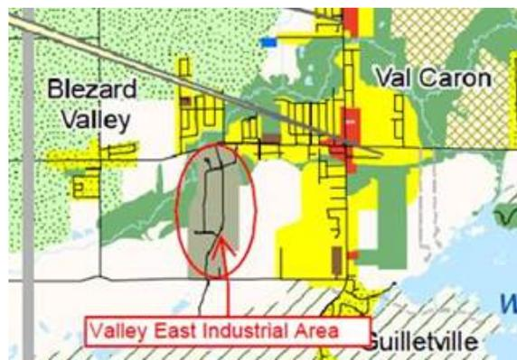
The only transmission connection alternative for this area is via circuit S5M. Supplying the new customer owned station will require the construction and a new 2km long 115kV tap. Adding 20MW on circuit S5M - a radial circuit out of Martindale TS - will lead to thermal overload on the Martindale TS autotransformer during certain contingencies and outage conditions.
