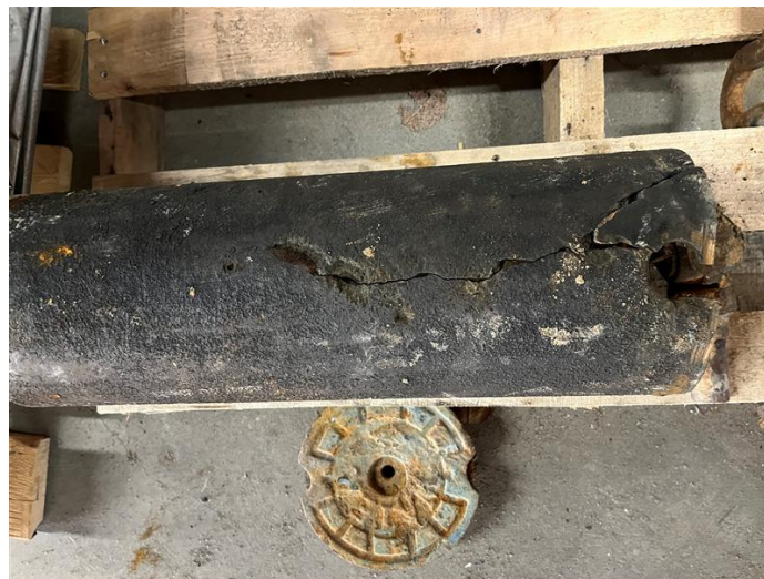
Figure 6 – First leak found using new leak detection technology. 1945, 150mm cast iron watermain.
