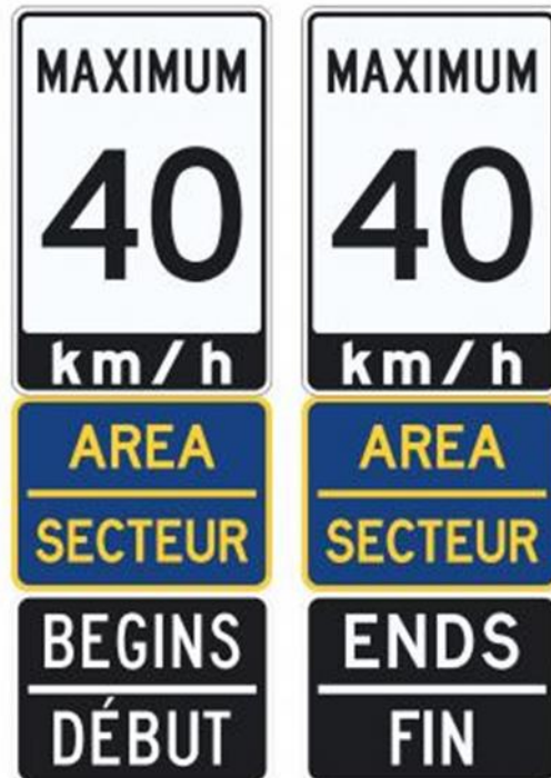
Figure 1 – Gateway Speed Limit Signs
