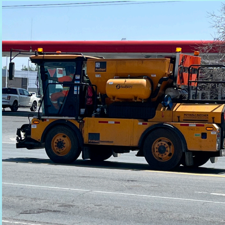
Began use of the Python 5000 pothole patcher
