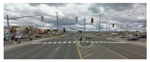
Pedestrian traffic signals manage the interaction between pedestrians and vehicles, and present operational benefits to pedestrians by providing priority over vehicles at all times. This priority may provide a sense of security for pedestrians, encourage pedestrians to cross at the controlled location and limit the number of locations where pedestrian crossings occur.
