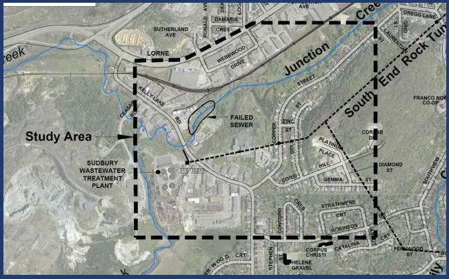
May 2007 – Junction Creek bank slope failure caused section of 600mm trunk sewer to fail; emergency repairs to slope and sewer; 2008 – structural liner
