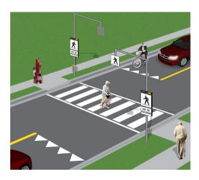
This system uses both the side mounted and overhead regulatory signs. This type of PXO is designed for medium volume, speed less than 60 km/h, single or multilane roadway, such as major collectors, arterial and high volume multilane roundabouts
