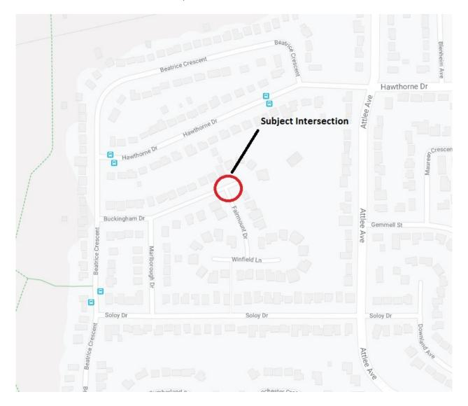
Fairmount Drive intersects Buckingham Drive forming a "T" intersection. Currently, the intersection is controlled by a Stop sign facing northbound traffic on Fairmount Drive. Traffic volumes are low at this intersection with adequate sight lines in all directions. A Yield sign is appropriate when the traffic volume is low, sight lines are good and stopping is not always Page 2 of 2
