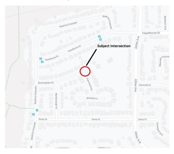
Fairmount Drive intersects Buckingham Drive forming a "T" intersection. Currently, the intersection is controlled by a Stop sign facing northbound traffic on Fairmount Drive. Traffic volumes are low at this intersection with adequate sight lines in all directions. A Yield sign is appropriate when the traffic volume is low, sight lines are good and stopping is not always
