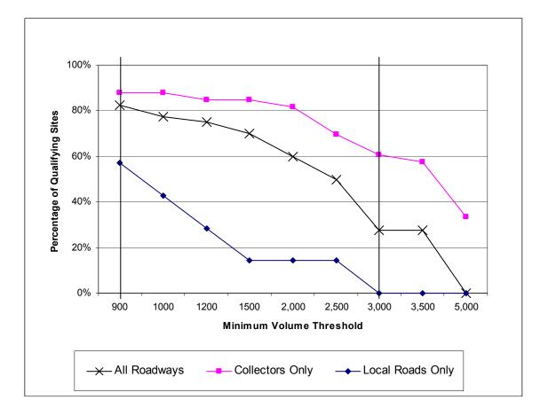
Exhibit 4-4: Pilot Testing: Volume Threshold Curves
