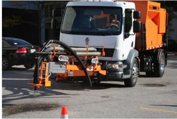
Figure 4 – All-in-one Spray Patcher (Transportation Association of Canada, Best Practices in Pothole Repair - 2019)
