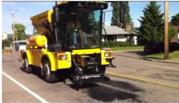
Figure 6 – Automated self-propelled pothole patcher (Transportation Association of Canada, Best Practices in Pothole Repair - 2019)
