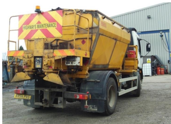
Figure 1 – Truck-mounted Hot Box (Transportation Association of Canada, Best Practices in Pothole Repair - 2019)
