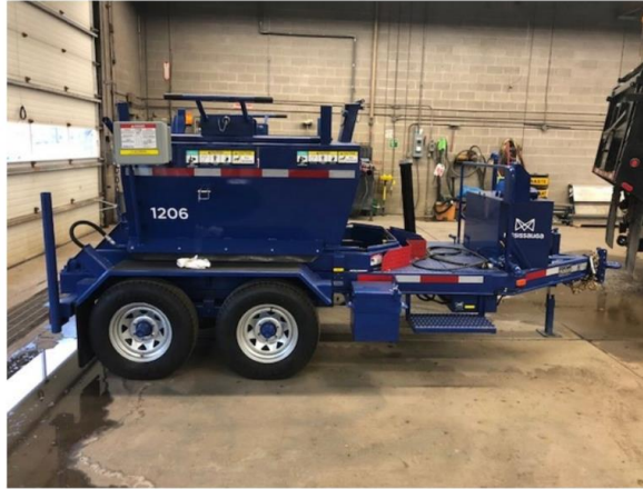
Figure 2 – Trailer-mounted Hot Box (Transportation Association of Canada, Best Practices in Pothole Repair - 2019)
