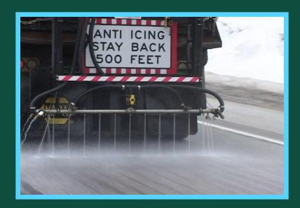
Deicing is the process of applying solids or liquids to a road to melt snow/ice
