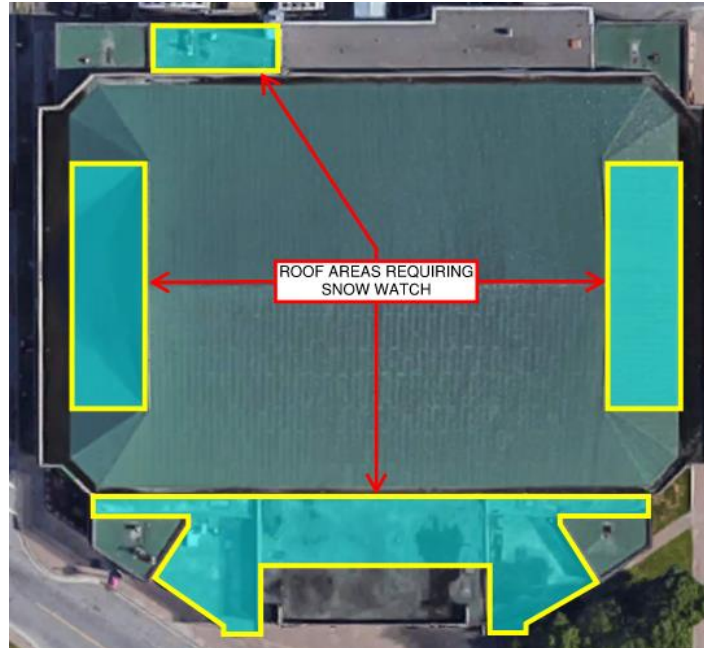
Figure 3: Sudbury Community Arena roof areas requiring snow watch.
